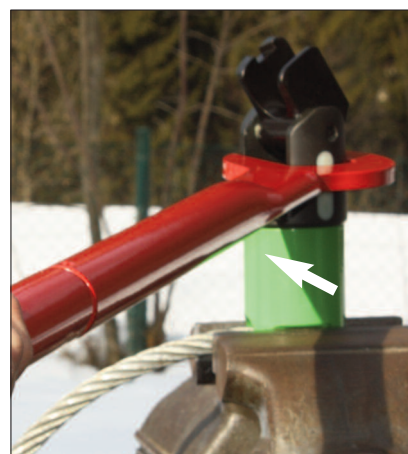
6a) Closing of cap in vice - clamp choker in vice - remount cap
