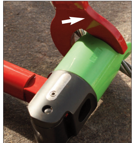
1b) Unscrewing of cap (on floor) Use both removal tools for opening. Turn cap in the direction of the arrow.
