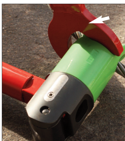
6b) Closing of cap on floor Use both removal tools for closing. Turn cap in the direction of the arrow.
