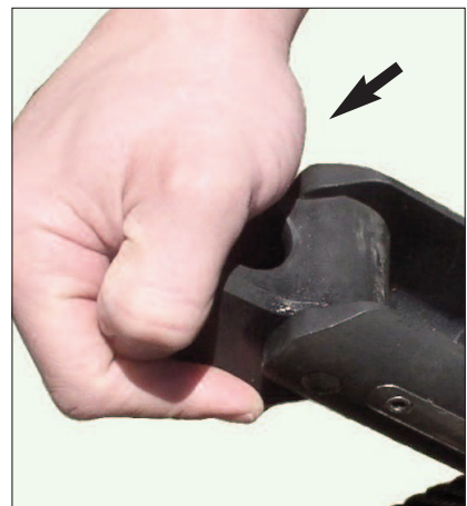
3) Cocking choker Press catch backwards until you hear the cocking mechanism engage.
