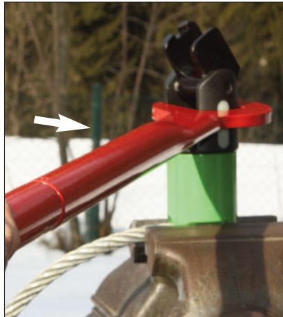
1a) Unscrewing of cap (in vice) - clamp choker in a vice - unscrew cap with removal tool
