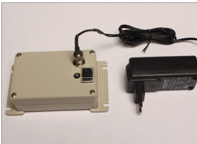
Repeater connected to charger unit
